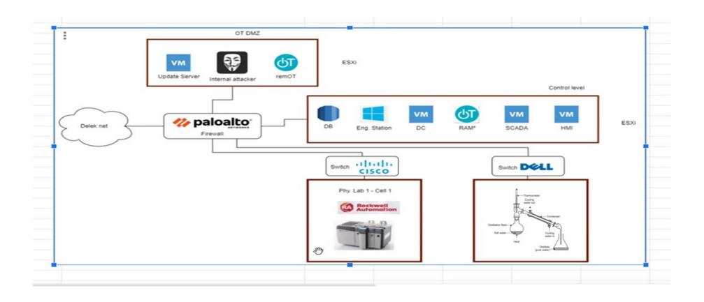
This is a Conceptual Process Control Simulation System for one individual process unit for one of the refineries, such as a Depropanizer, which is a type of distillation unit that removes propane from liquids. The Simulated Distillation system will be able to sit on a normal work desk and will be no bigger than 2ft in width.
