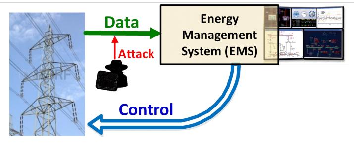
Knowing system configuration, attacker can maliciously change a subset of measurements with counterfeit data before they reach the EMS
