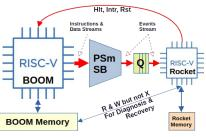
GaTech will designs PEMon to showcase a new capability for program execution monitoring at instruction level granularity, without impacting the performance of the monitored processor. PEMon opens a new opportunity for detecting and mitigating low-level events and attacks that are either too expensive and/or too faint for software to monitor and detect.
